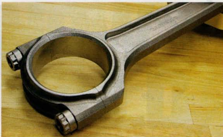
Measuring 6.800 inches, the Carrillo steel rods were designed in collaboration with ERL to provide sufficient cam and block clearance.
