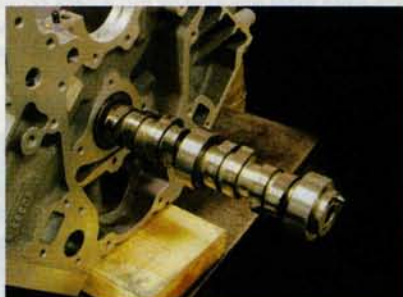
Since the goal was to build a streetable motor that represented what many enthusiasts would probably build, SAM installed a conservative Comp 248/254-at-0.050 hydraulic roller cam with 0.647-inch lift. It was ground on a small base circle for additional rod clearance. With slightly more duration, SAM says the combination would easily put out an additional 50-60 hp.
